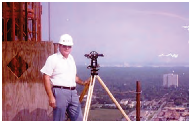
The author in the early 1970s doing STL path survey work in connection with the Houston One Shell Plaza master FM installation.
