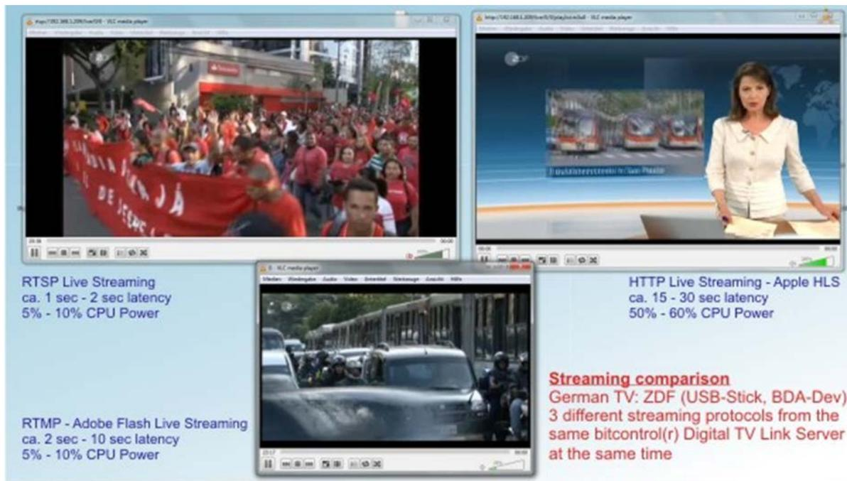
Figure 3: Performance comparison of 3 different streaming protocols (RTMP, HLS and RTSP)
