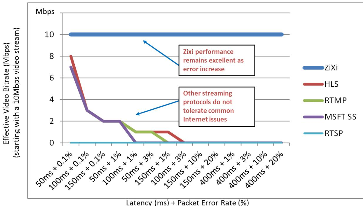
Figure 4: Zixi technology performance compared with many of the popular streaming protocols with increasing latency and packet loss
