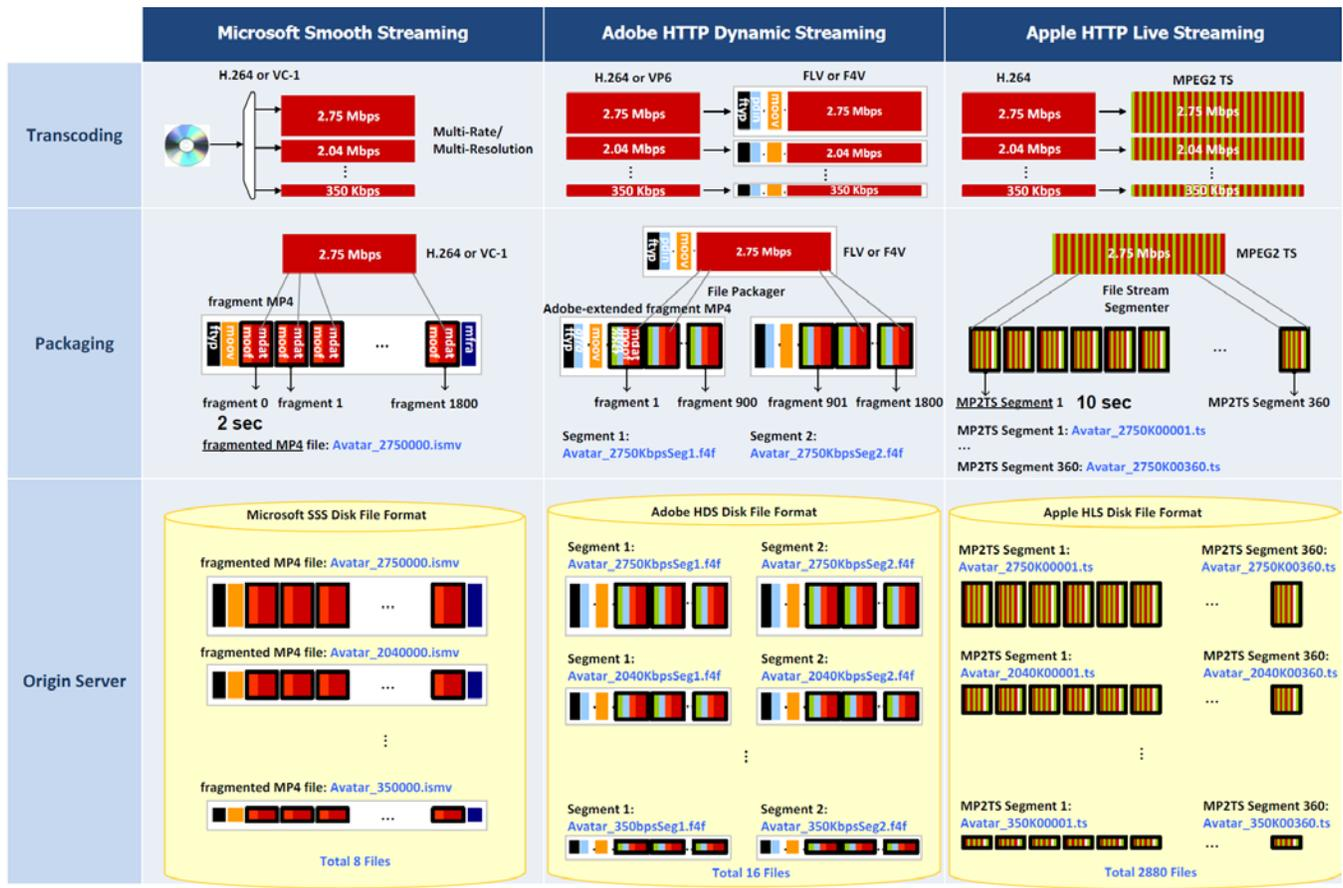
Figure 2: HTTP Adaptive Streaming comparison
